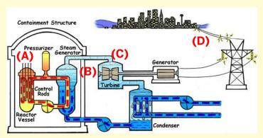
Power plants create electricity by running steam turbines, which are powered either by fossil fuels – coal, oil, natural gas – or by nuclear power. Nuclear technology produces energy by splitting uranium atoms in a process called fission. (A) Fission generates heat in the reactor vessel that (B) boils water for the steam that runs the (C) turbines, which produce the (D) electricity that we all use.
